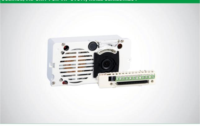
Audio-video unit for ViP system including terminal block complete with front-adjustable mini lens colour camera, LED camera lighting. Complete with terminal block and digital audio management system with Echo-cancelling, watertight loudspeaker and electret microphone, loudspeaker volume adjustable from the front. For fitting in modules: part. 33410, 33411 and 33412. Dimensions: 102x55x38 mm.
