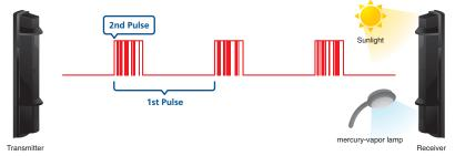
The SL-QDM and SL-QDP series offer double modulation beams that differ in pulse patterns. This can enhance signal discrimination against potential noise interference such as sunlight or other external light sources, resulting in a reduction of missed or false alarms. Together with OPTEX triple layered Sunshine Protection Technology, it ensures high reliability under the severe outdoor security environment.
