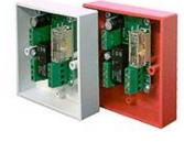
The unit has a wide ranging trigger **INPUT** voltage (9.5V to 42VDC and 7.5V to 30VAC RMS) and also incorporates a timer (this counteracts fire control panel interlink latchups – enabled by removing the LINK). A series diode is also "built-in" which allows easy connection to fire alarm monitored bell type circuits.
