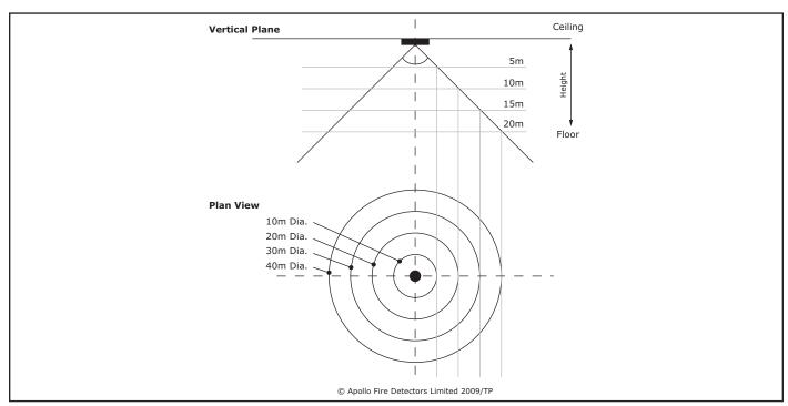
Fig. 2 Ceiling mounting example
