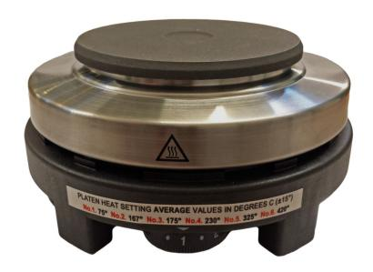
Patols Infrared Heat Platen is used to test and commission the 5000 series detectors. The platen uses a rapid controllable thermal energy that provides no visible sign of heat, by producing black body Infrared emissions.
