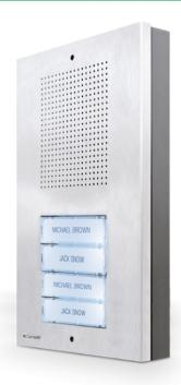
Extra series audio entrance panel with stainless steel cover and nameplate backlighting. To be completed with single button art. 9211 (pack of 4 units) to offer 4 call buttons, or with double-height button art. 9210 (pack of 2 units) to offer 2 call buttons. The entrance panel can be surface-mounted or flush-mounted using the relevant accessories supplied. Traditional 4 + N wiring system. Dimensions (W x H x D): 95x165x6.5 mm (flush) - 25 mm (surface).
