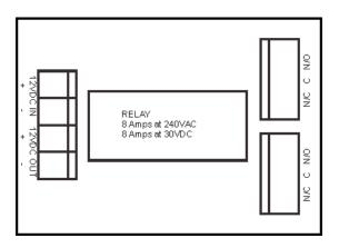
Note: Polarity must be correct for the relay to activate.
