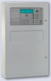
The HS-5800 series of control panels are fully expandable from 2 to 8 loops and supplied with 8 on-board sounder circuits, 20 programmable zonal LED's with slide-in labels, and 25 system LED's for information purposes. There are also 8 programmable function buttons with LED indication for confirmation of operation.
