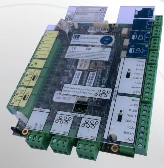
The i-Net PLUS Intelligent Door Controller from Controlsoft provides a single board solution for interfacing one or two doors to a Controlsoft Identity Access system. In addition, other i-Net PLUS controllers, I/O Expansion Boards and RS485 Readers can be added on the i-Net PLUS RS485 ports to expand its capabilities.
