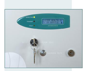
The interface to the host Fire alarm system comprises of multiple prioritised Fire inputs and a further input to provide for fault indication from the Fire panel. For ease of installation, a monitored interface cable is provided with the system which also includes a "common fault" relay output back to the host Fire alarm panel. This will activate if the PageTek Pro suffers a mains failure, transmitter fault, antenna mismatch, link failure, low battery or missing battery condition.
