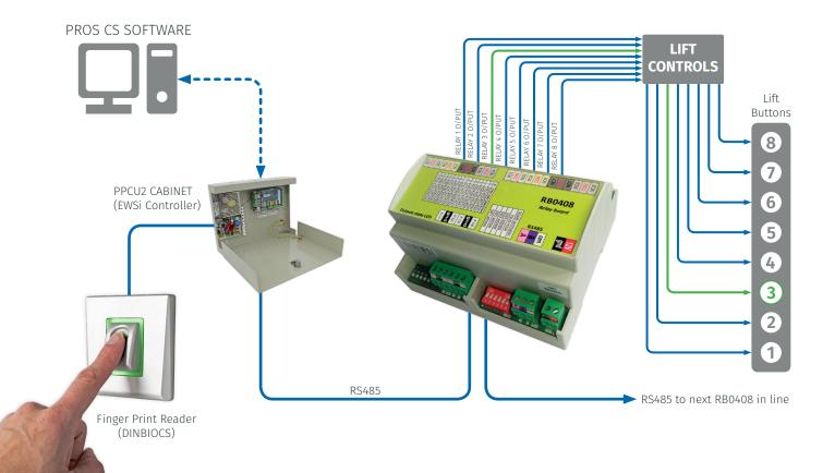
Program and configure the RB0408 interface relay using the PROS CS software.
