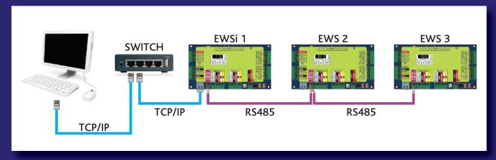
Combine both TCP/IP and RS485 on the same system for maximum flexibility.
