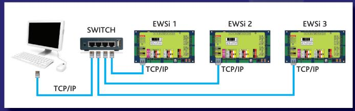
Distribute controllers via a TCP/IP network up to 100m from switch/router.
