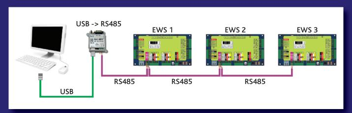
Connect up to 31 controllers via an RS485 bus over a distance of up to 1km. Use RS485 hubs and repeaters for larger distances or additional controllers.
