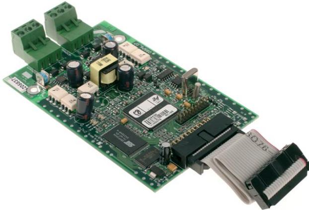
The VESDAnet<sup>™</sup> Interface Card (VN Card) is a simple interface card for the range of VESDA LaserFOCUS<sup>™</sup> (VLF) smoke detectors. The VN Card provides seamless VESDAnet communication from the detector to other VESDAnet devices, including configuration and monitoring tools.
