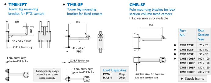
All brackets for camera mounting have a Ø127 mounting plate with 8 no Ø8.5 equi - spaced on 101.6 PCD
