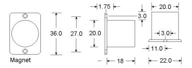
The YA40 is a universal fully sealed Flush Contact with magnetic shielding. It meets all of the necessary requirements for magnetic contacts permitting it to be used within Grade 3 installations. The contact has installer selectable End of Line (EOL) and alarm contact bypass resistors, and benefits from the option of a second device connected in series.
