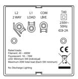
Remove the existing light switch, and transfer the wires to the ZV700B according to the following instructions;
