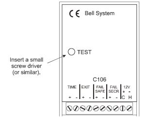
◆ Finally the red and green LEDs will flash together for 1 seconds and extinguish. The Factory Settings are now restored; release the TEST button.
