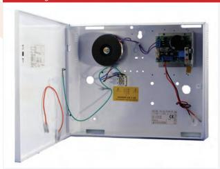
A Range of Power Supplies available in a variety of outputs housed in metal enclosures with a detachable hinged lid. Available in 1, 2, 3 & 5 Amp, the EMMX Range is a Multi Indicator (Mains On & Fault) Power Supply. The outputs are full current to load and are exclusive of the battery charging facility.
