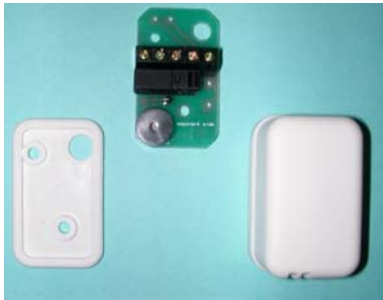
Fig. 3 - Z20 Final Exit Set Switch
